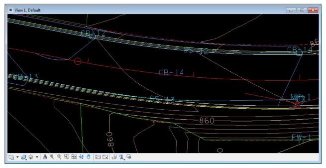
**NOTE:** Be sure to toggle **Use MS Element** <u>OFF</u> for subsequent Links that are not curved. When used, the Link position and length are defined by the MS Element. **Caution must be used** in order to properly define the Link.
