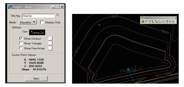
The Microstation Change Element Fill Type tool can be used to illustrate the ponded water for visual analysis. Use the Change Attributes tool to change the color to blue if desired.
